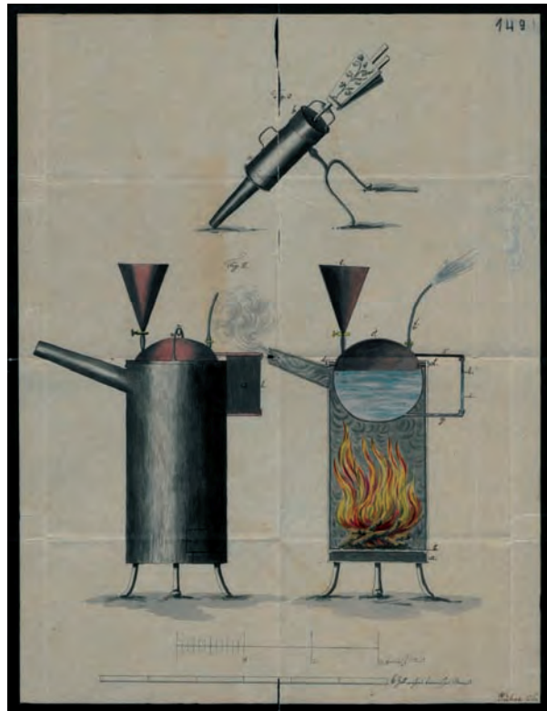
Fig. 9 Gottlieb Kühne, renderings of fumigator (above), and steam-producing boiler (below), 1825 (GStAPK, BPH, Rep. 192, Nachlass Lenné, Nr. 4, Bl. 149)
